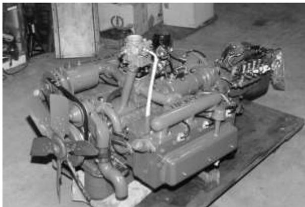
modified 6 ALV 335 engine produced 166 horsepower and delivered an astounding 372 foot-pounds of torque. From a stand still, the engine could provide enough power in first gear to strip teeth off the transmission. Tests later proved that Preston Tucker had an extremely well-proportioned power plant and drive train.
