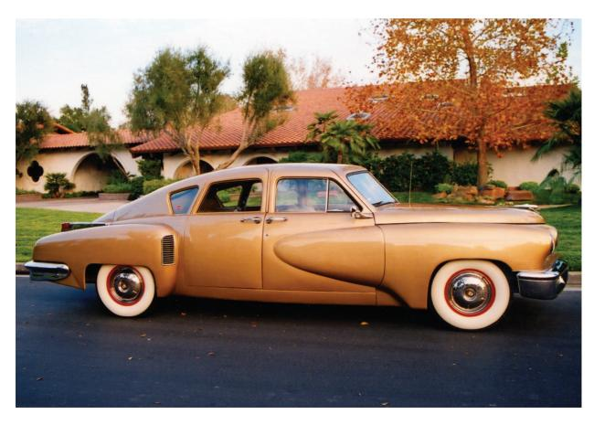
California, the new owner obtained a 335 ALV Franklin engine from a test chassis and a Cord 812 transmission. Additionally, a welder was hired to install the front engine hanger to match the Cord gearbox, while an upholsterer provided the interior and other components such as the control cables from test car no. 1027 that rolled at Indianapolis. A new instrument panel became the final component required to make the car roadworthy.
